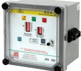
Whenever there is a ground fault in one phase, the voltage in other two phases will rise and generate a sensing voltage which is continuously monitored in the relay. When this voltage exceeds the set value the internal relay operates. The Relay contacts can be used for Alarm & Trip purpose.
